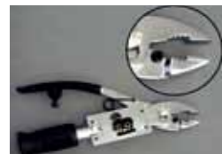
Small type [JPS100Y] Length 200mm Weight 300g Aperture 10~12mm Maximum about 20mm
